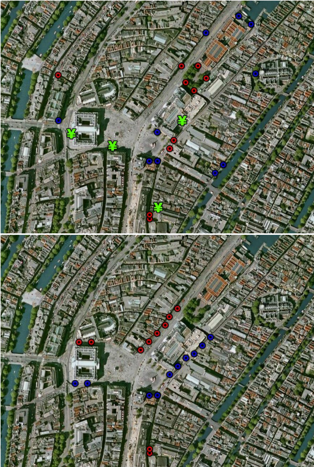
Figure 63: The locations of the wells for the mixed case (above) and for the grouped case (below). Warm wells are plotted with a red circle and cold wells with a blue circle. Monowells are plotted with a green Y.
