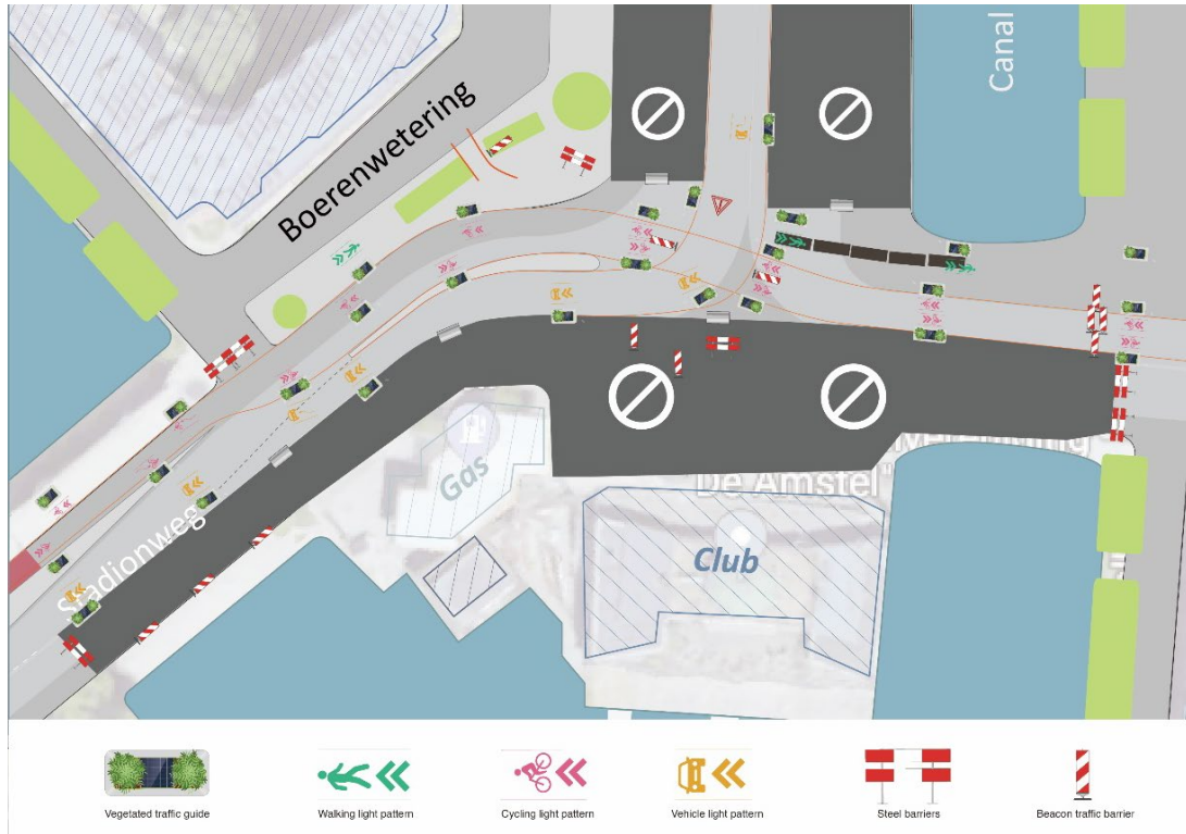
Figure 29. Vegetated traffic guide in roadwork space arrangement
